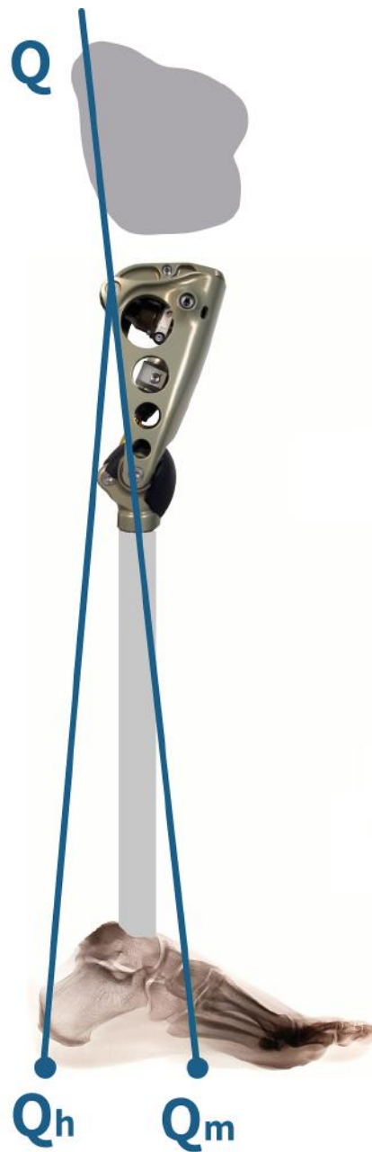
Figure 3.3: The Q-line in the VGK-S alignment
