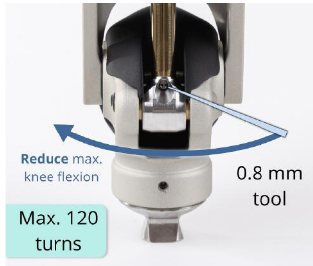
Figure 5.1: Adjustment of the maximum knee flexion
